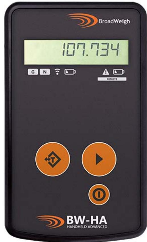
The device features a backlit display, which makes it usable in low-light environments. Broadweigh wireless handheld display BW-HA is powered by a pair of standard alkaline AA batteries and is configured using free BW-Toolkit software which runs on a PC connected to the BroadWeigh base station.
