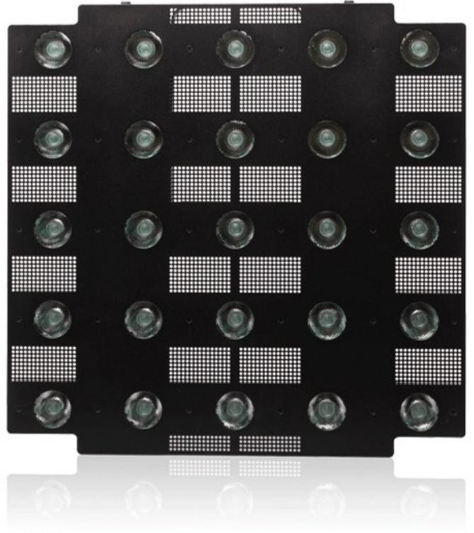
The CHROMAPIX 55 is a Pixel Mappable RGBW LED unit which utilize 25 x 10W RGBW LEDs that are configured in 5 x 5 pixel matrix to create spectacular 3D beam projections in a tight beam angle for maximum throw effects.
